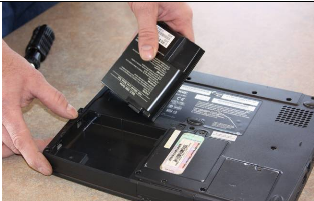
1. Laptop HD: Remove any power cables and battery.
