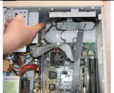
3. Locate and disconnect the circuit connectors.
