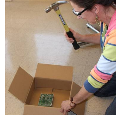
8. Wear glasses, use hammer to destroy circuitry and warp the platters inside.
