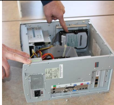
2. Remove casing and locate hard drive (touch metal frame before reaching in).
