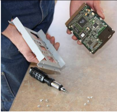
7. Remove any screws and separate the hard drive from its casing.
