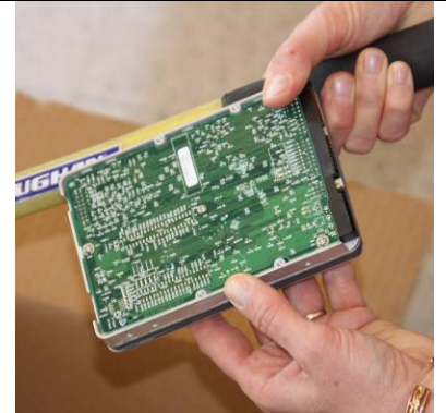
9. A few dents in the HD circuit board will render the unit inoperable.
