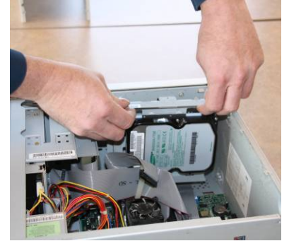
6. Slide out the hard drive and casing.
