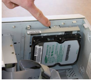
5. Remove screws holding HD in place.
